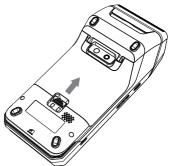
SAM and SIM1,SIM2 are identified by the engraved marks on the lower housing.
